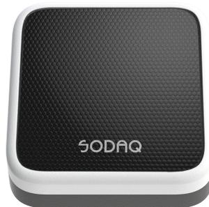
It is recommended to use **2 strips of 3M Tape (VHB or GPH)** - or alternatively **LSE series tape** for applying to some plastics like HDPE - each **5.0 x 1.9 cm** long attached to the back of the tracker as shown in the image below. It is important that the device is attached to a smooth, non-curved and clean surface on your asset. The surface should be at least **80x80 mm**.
