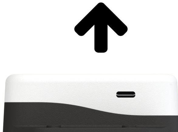
If a horizontal orientation is not feasible, a **vertical orientation** is the second preference. Note that with this orientation, GPS positioning accuracy can diminish in comparison to a **horizontal orientation**.
