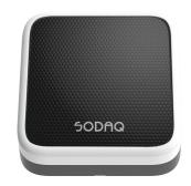
It is recommended to use 2 strips of 3M Tape (VHB or GPH) - or alternatively LSE series tape for applying to some plastics like HDPE - each 5.0 x 1.9 cm long attached to the back of the tracker as shown in the image below. It is important that the device is attached to a smooth, non-curved and clean surface on your asset. The surface should be at least 80x80 mm.
