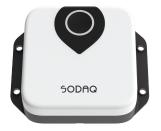
It is recommended to use **non-countersunk pan head M4 screws or bolts** when mounting a flanged TRACK to an asset.
